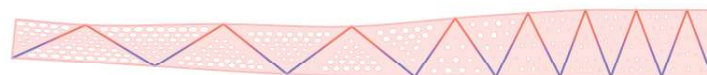
Fig.3 Longitudinally differentiated elasticity of the wall. Silicone shown in pink and metal frames in grey, while red and blue show the charged state of the electromagnets
