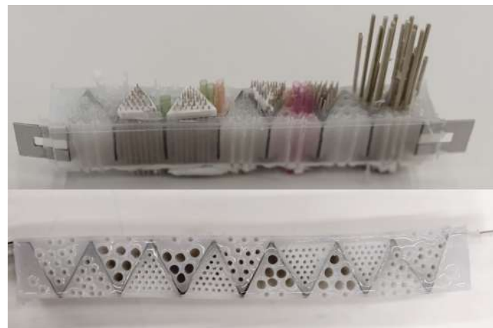
Fig.5 The three different perforating cylindrical elements and the resulting porous prototype
