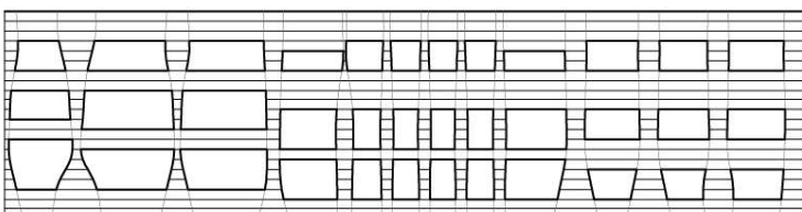
Fig.10. Auxetic system: elevation sample showing the lofted geometry in line with 3D-printing layers and circle variation
